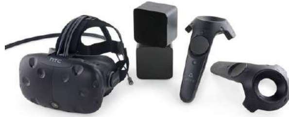
Figure 5.1: The components of the HTC Vive setup: the headset with integrated screen, the base stations positioned in the room that track the sensors, and two controllers that have both button and position tracking.
