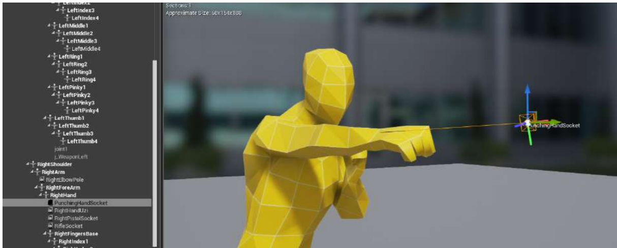
Figure 2.5: The IKinema system in Unreal Engine with the fist trying to follow its target transform.
