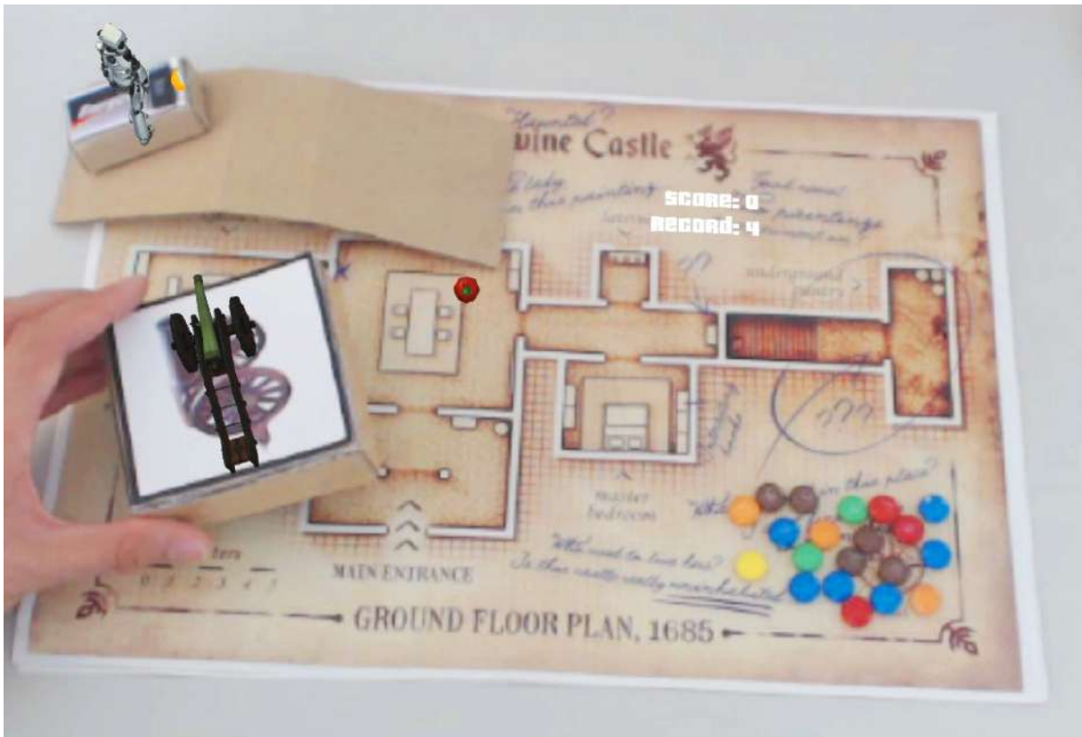
Figure 6.11: A screenshot from the latest demo. The droid can be seen while it keeps balance from being hit with a banana shot from the cannon. The cannon is spawned on top of the cardboard marker and can be oriented to hit the character. It is also possible to see a cardboard ramp in the real world, which the droid can climb as the ramp is brought into the virtual world and made interactive. An uneven terrain with candies can also be seen. The droid can walk on this terrain and keep balance although the terrain isn't flat.
